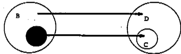
Fig. 4. Inheritance Case III. A \subset B . F_A \subset F_B . C \supset D . F_C \subset F_D . Only the feature sets of the respective concepts are shown here. One arrow is drawn in place of pairwise connections.
